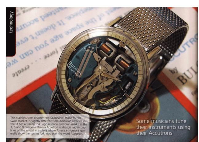
"Early Accutrons looked like typical watches and sported gold dials. Bulova wanted jewelers to be able to show their customers how different the Accutron was inside, so the company made display models with the dials removed, allowing people to view the watch's internal parts, including the tuning fork and electronics," says Piker.
